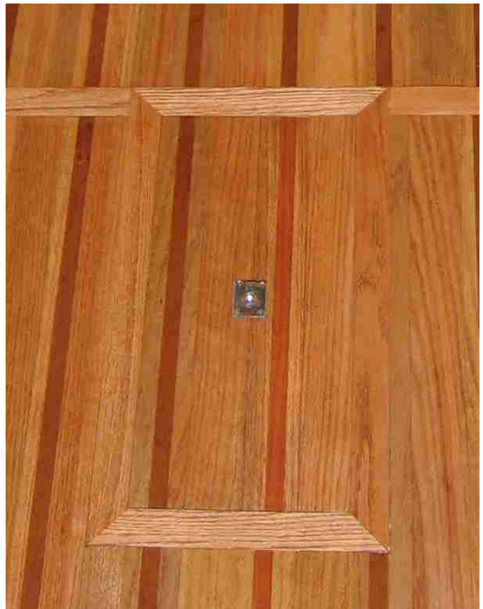
Photo 4 Bilge Cover and Frame
